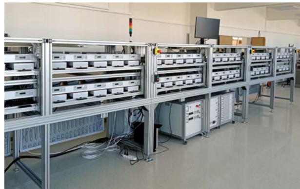
Electricity Meter Test Equipment ELMA with horizontal meter placing - fully automatic (customized, horizontal meter placement)
